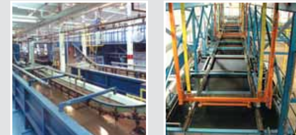
Typical autodeposition equipment layout for hoist operations
