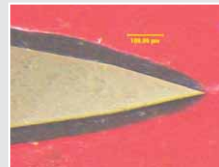
Scanning electron microscopy (SEM) photo shows a consistent coating thickness around the edge of a razor blade
